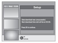
To download GUIDE Plus+ data, turn off your unit at the time displayed on the screen or download the data manually from "Data Download" in the Setup menu at that time. (+ 23, Changing the settings)
